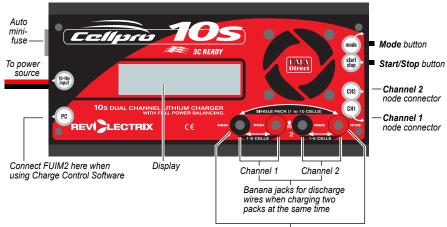
Banana jacks for discharge wires when charging one pack, or insert Plug Blocker when not charging through discharge wires
